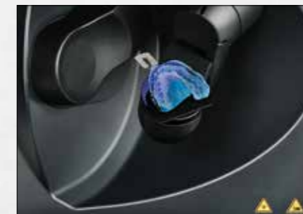
Impression scan. The inEos X5 scans many different shapes and sizes of impression trays with no difficulty.
